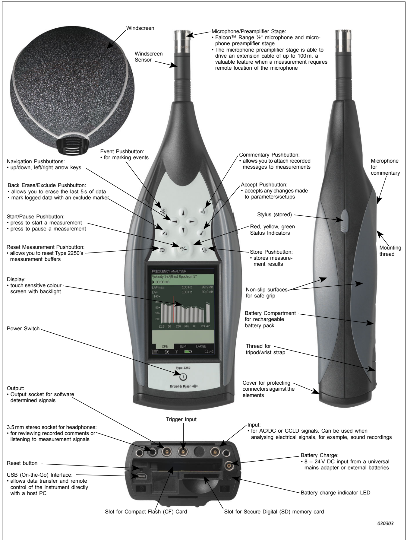
Fig. 1 Key features of Hand-held Analyzer Type 2250
